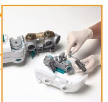
Rotate the breathing circuit module counterclockwise and separate the two sections by pulling them apart.
